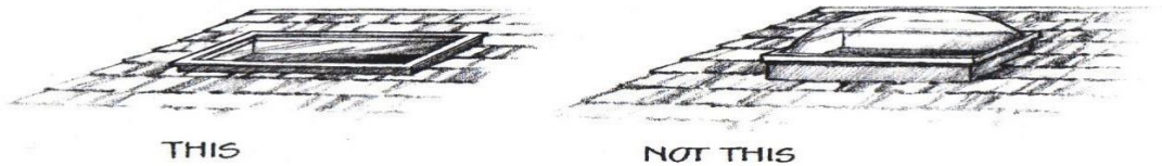
SKYLIGHTS (Figure 3.K)
